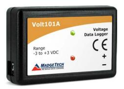
MadgeTech's Volt101A data loggers are versatile data logging devices with many uses and applications. Connect negative and positive wire leads directly to the terminal port on the Volt101A to monitor and measure voltage levels. The Volt101A is commonly used to assess battery efficiencies or photovoltaic studies to identify how much energy is being created from solar cells.
