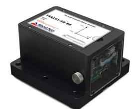
The TSR101-EB is a battery powered, stand alone transient tri-axial shock recorder. The TSR101-EB measures and records instantaneous shock levels when the user-selectable shock levels have been exceeded. There are 15 rates to chose from ranging from 1024Hz to 1 Hz. The TSR101-EB is valuable in characterizing environments such as railcar coupling impacts and aircraft turbulence monitoring.
