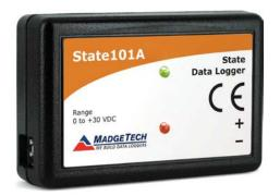
The State101A data logger monitors and records the occurrence, duration and status of predetermined events by measuring changes in voltage. Typically connected to a relay or switch, this data logger features a removable screw terminal block to easily disconnect and retrieve the logger for data download without disrupting wiring connectivity.
