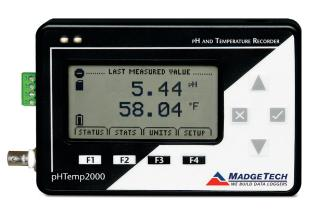
pHTemp2000. Temperature compensation is automatically done internally to the unit.
