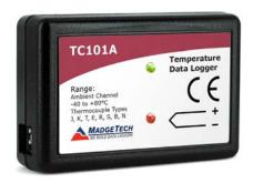
The TC101A temperature data logger is a compact versatile device to be used with thermocouple probes for accurate temperature monitoring and profiling. This data logger is an ideal and affordable solution for applications such as HVAC studies, oven profiling, dry-ice shipments, process validation and many general purpose temperature monitoring applications.
