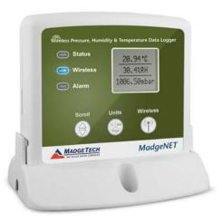
This data logger allows users to select the desired units in which the data is displayed. The RFPRHTemp2000A has a wide range of units available for each channel: °C, °F, °R, K for the temperature channel, %RH, mg/mL, Dew Point for the humidity channel and mbar, PSI, inHg, mmHg, atm, Torr, Pa, m, kPa, MPa for the pressure channel. The unit is available for display on the LCD screen as well as in the software.
