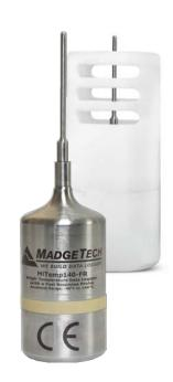
The Trigger Settings feature of the HiTemp140-FR allows users to configure high and low temperature thresholds that when met or exceeded, will automatically start or stop recording data to memory. This data logger is capable of storing up to 32,700 date and time stamped readings and features a nonvolatile solid state memory which retains data even if the battery becomes discharged.
